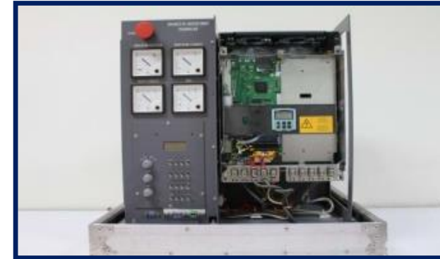
TWO SET OF SINAMICS 6RA80 2 X DC DRIVES & 2 X DC MOTORS (Batch of 6 to 8 x Students per DRIVE )
